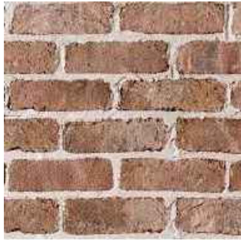
FB1 FACE BRICK - RECLAIMED RED BRICK OR SIMILAR TO U1, U3 & U4 SELECTED GF WALL, PORCH AND LETTER BOX PIERS
